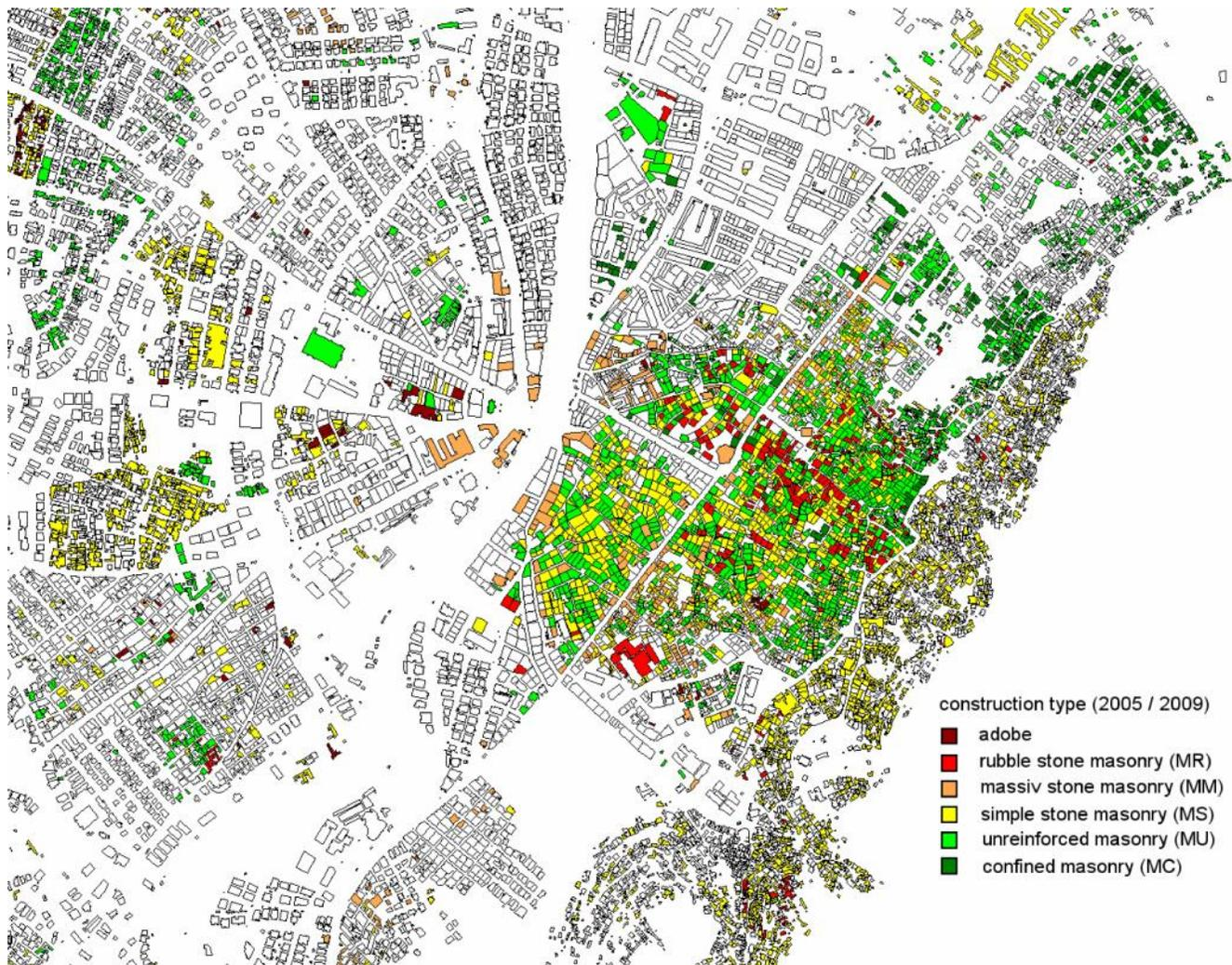
Figure 2. Masonry building types in Antakya (Turkey) based on the building stock surveys in 2005 and 2009
