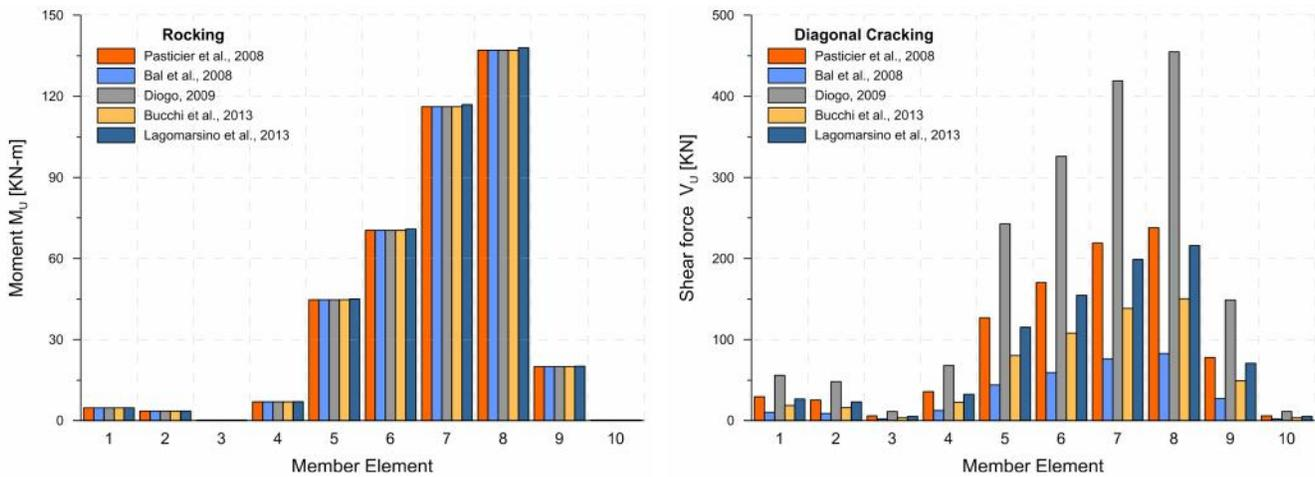
Figure 6. Comparison of non-linear hinge models for masonry piers: failure type rocking and diagonal cracking
