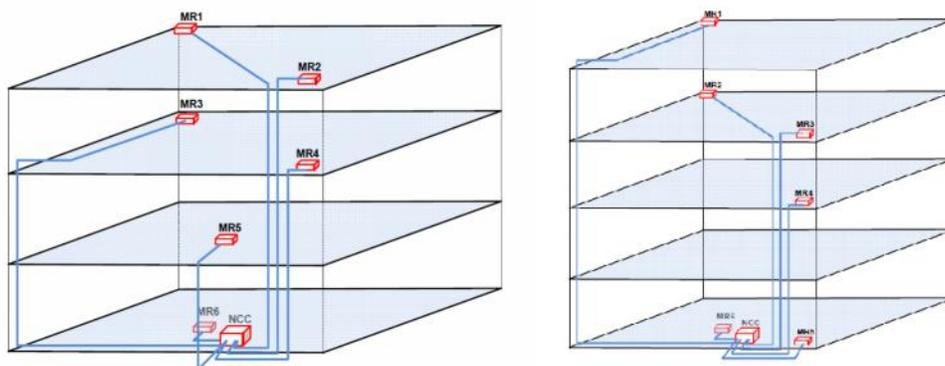
Figure 5. Example schemes of the temporarily ambient vibration measurements; Note: The location of the sensor strongly depends on the accessibility.]
