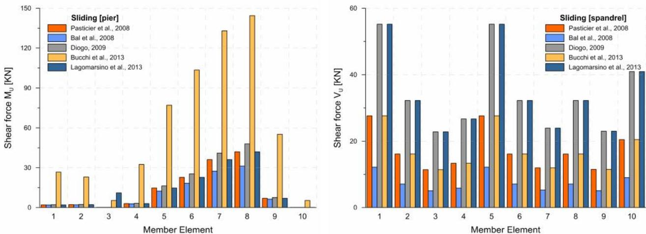
Figure 7. Comparison of non-linear hinge models for the failure type sliding for the masonry piers and spandrels
