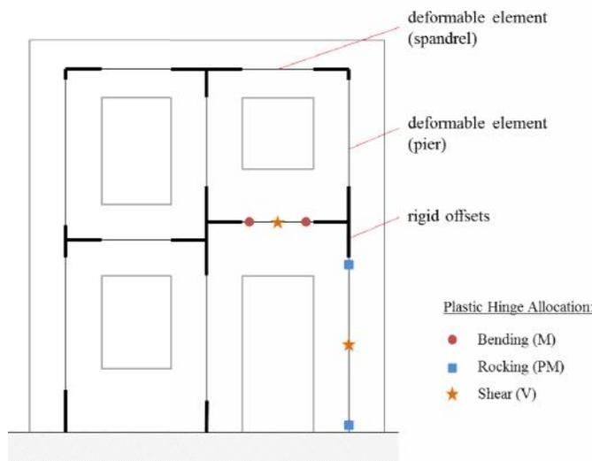
Figure 1. Scheme of the Equivalent Frame Model and the assignment of plastic hinges
