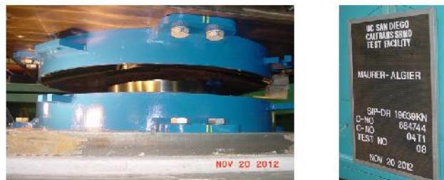
Figure 10. Prototype isolators installed into CALTRANS test rig in San Diego
