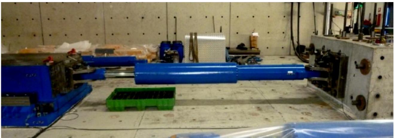
Figure 13. Original hysteretic loop of tested MHD for 1,000mm/s velocity [9] on left-top; CE mark on right top; damper test at EU Center Pavia on bottom;
